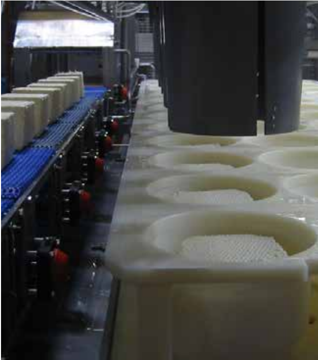
Filling of pre-pressed cheeses. Simultaneous filling of more than one cheese depending on the capacity requirements of the processing line.
