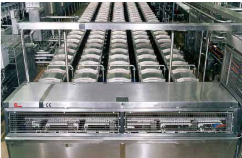
Pressing takes place in closed tunnels by means of a diaphragm pressing on the entire surface of the mould lid.
